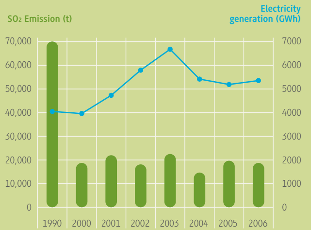
Figure 7: Pollutant emissions to air from HEP's thermal power plants - SO 2
